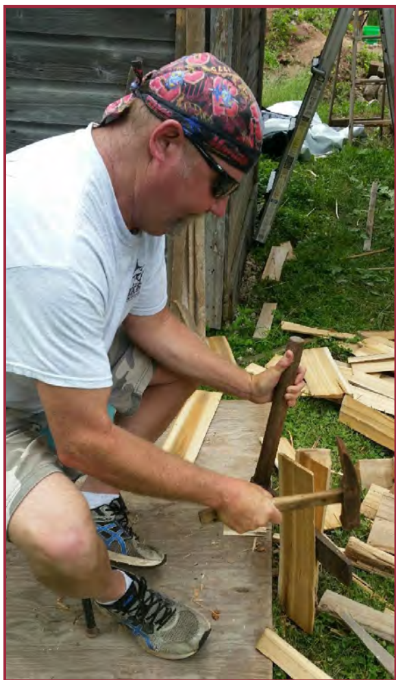
President Richard Lutze uses a froe to create a cedar shingle. You can learn this skill yourself on August 19 in the Old Time Trades Workshop from 9:30-11:30 a.m. See centrevillesettlement.com for details.
