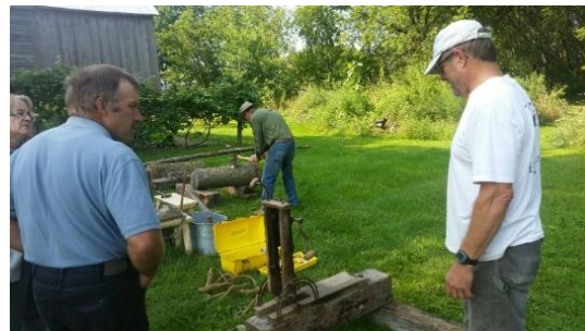
Chris Kuehnelt explains how the boring machine makes a series of 2" holes to create a mortise for timber framing
