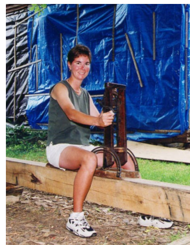
Boring machine for drilling holes in timbers. Original tool. Lynn Kalista
